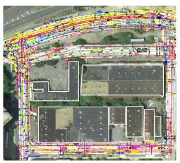
Figure 2 – Original Site with Existing Utility Overlay
