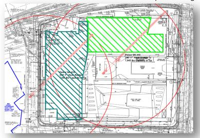
Figure 13 – Horizontal Crane Plan Courtesy of Facchina Construction Company
